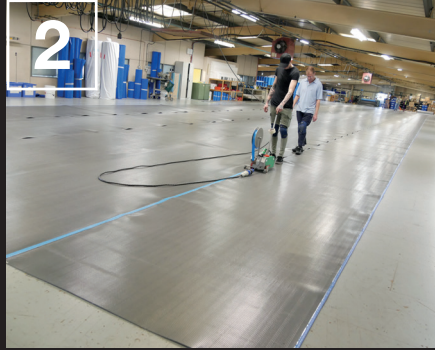
Step 2. Welding the cover together A hot air welder is used to join the seams together. The material is welded on both the laminate and foam sides. Once welded the cover is cut to the exact measurements.
