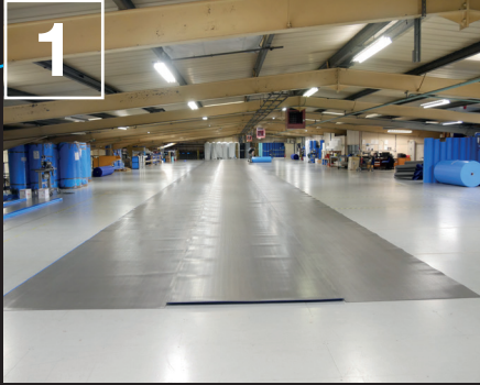
Step 1. Measuring and laying out the cover material 5mm Supercover material is cut to suit the length and width of the pool.
