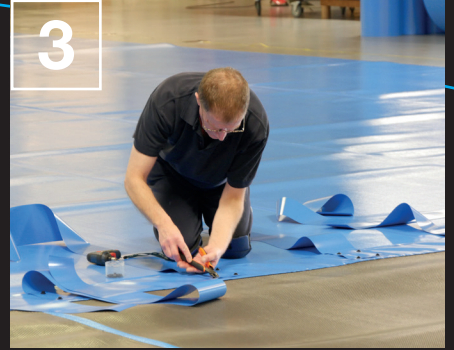
Step 3. Fitting the straps Hard wearing tarpaulin straps are attached to the cover at even spaces.
