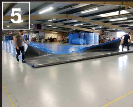
Step 5. Checking the cover Once complete the cover is turned over, checked for size and quality inspected.
