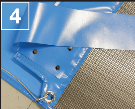
Step 4. Detail of the straps & wind wires 4mm stainless steel wire is hemmed into the entire length of the cover so it can be secured around the pool.
